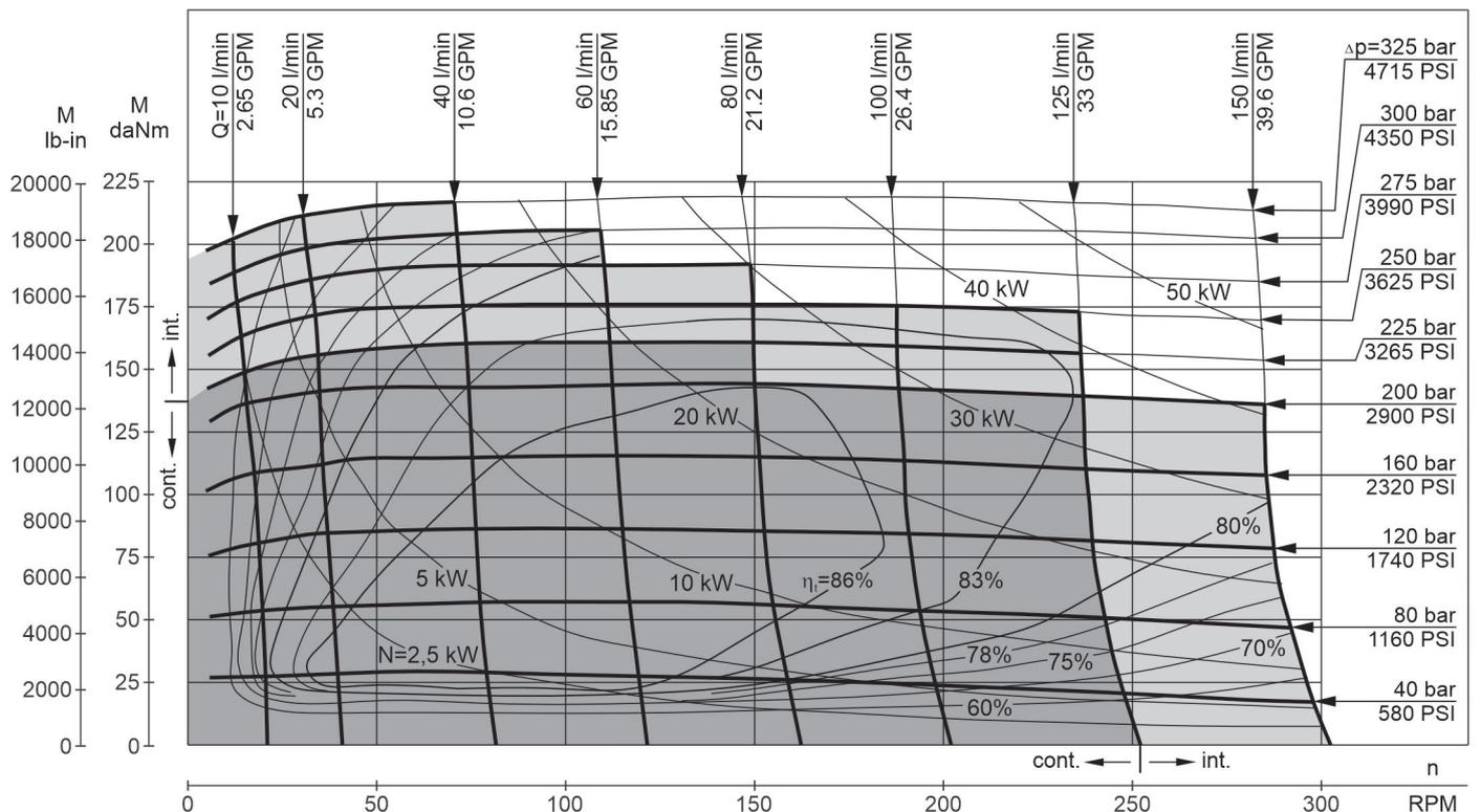
The function diagrams data is for average performance of randomly selected motors at back pressure 72.5÷145 PSI [5÷10 bar] and oil with viscosity of 150 SUS [32 mm<sup>2</sup>/s] at 122°F [50°C].
