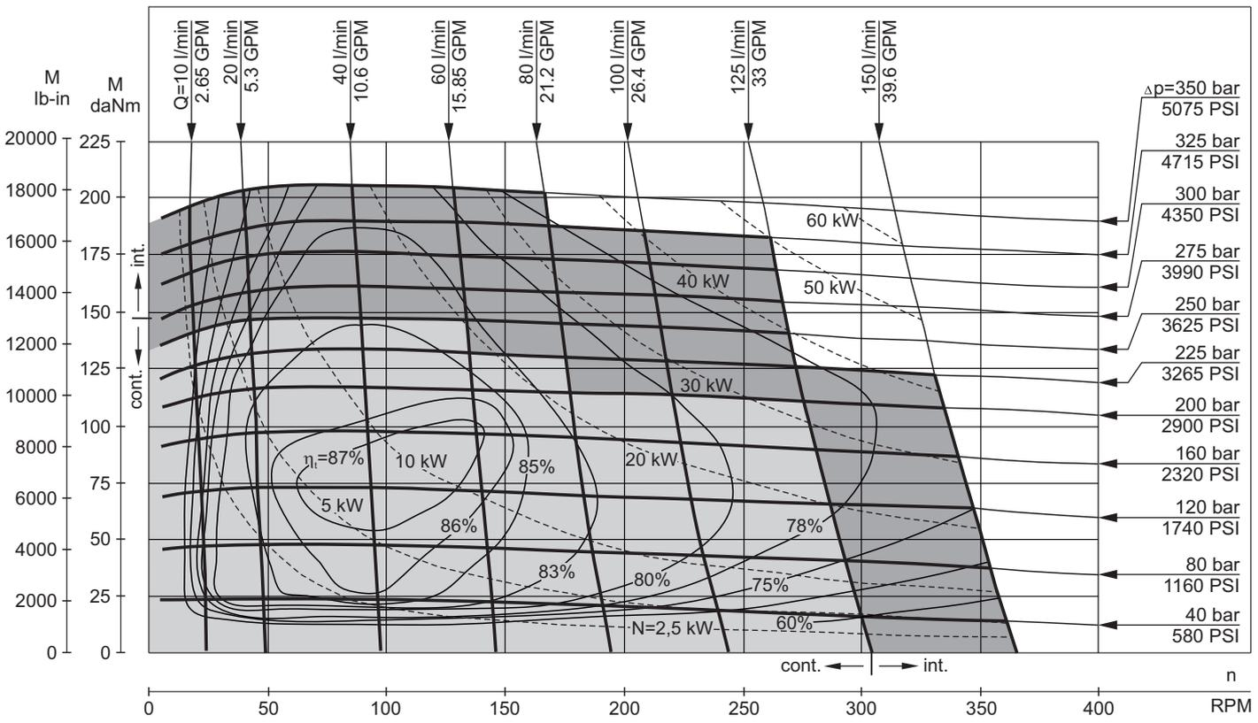
The function diagrams data is for average performance of randomly selected motors at back pressure 72.5 PSI  $\pm$  145 PSI [5  $\pm$  10 bar] and oil with viscosity of 150 SUS [32 mm<sup>2</sup>/s] at 122°F [50°C].
