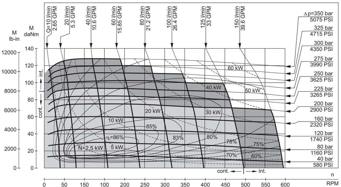
The function diagrams data is for average performance of randomly selected motors at back pressure 72.5 PSI  $\pm$  145 PSI [5  $\pm$  10 bar] and oil with viscosity of 150 SUS [32 mm<sup>2</sup>/s] at 122°F [50°C].
