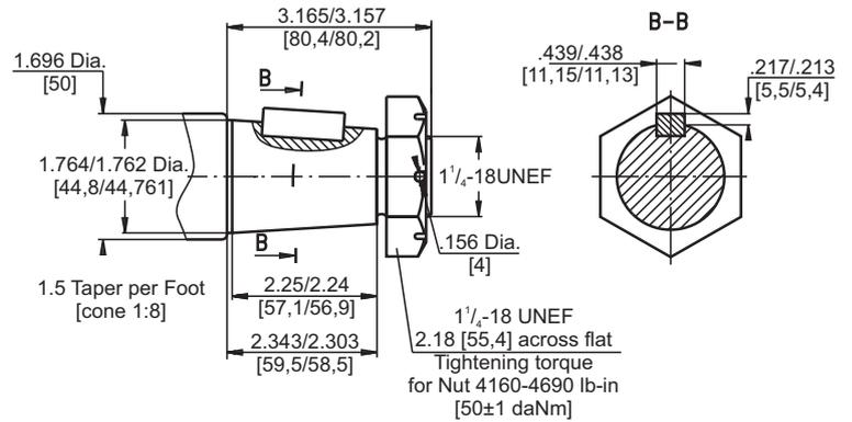
Requirement max. Torque must not be exceeded.
