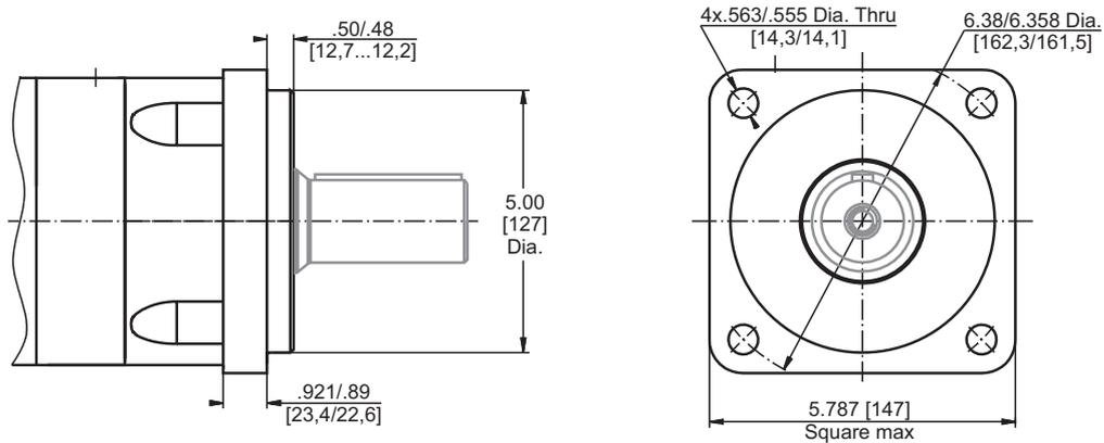
**W** 4-Bolt flange, Wheel Motor
