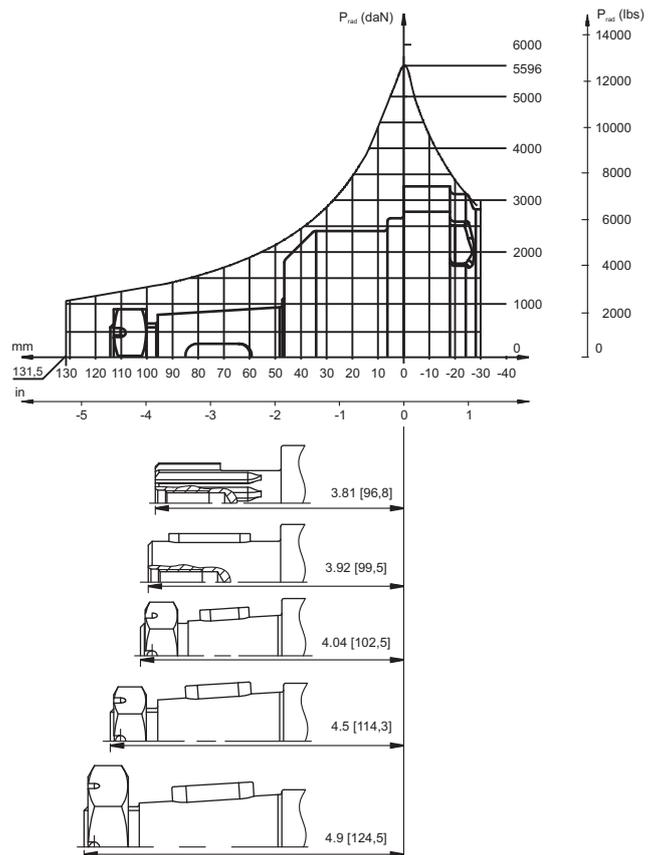
**MAX. PERMISSIBLE SHAFT SEAL PRESSURE for MTK motors**
