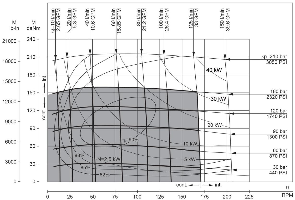
The function diagrams data is for average performance of randomly selected motors at back pressure 72.5÷145 PSI [5÷10 bar] and oil with viscosity of 150 SUS [32 mm<sup>2</sup>/s] at 122°F [50°C].
