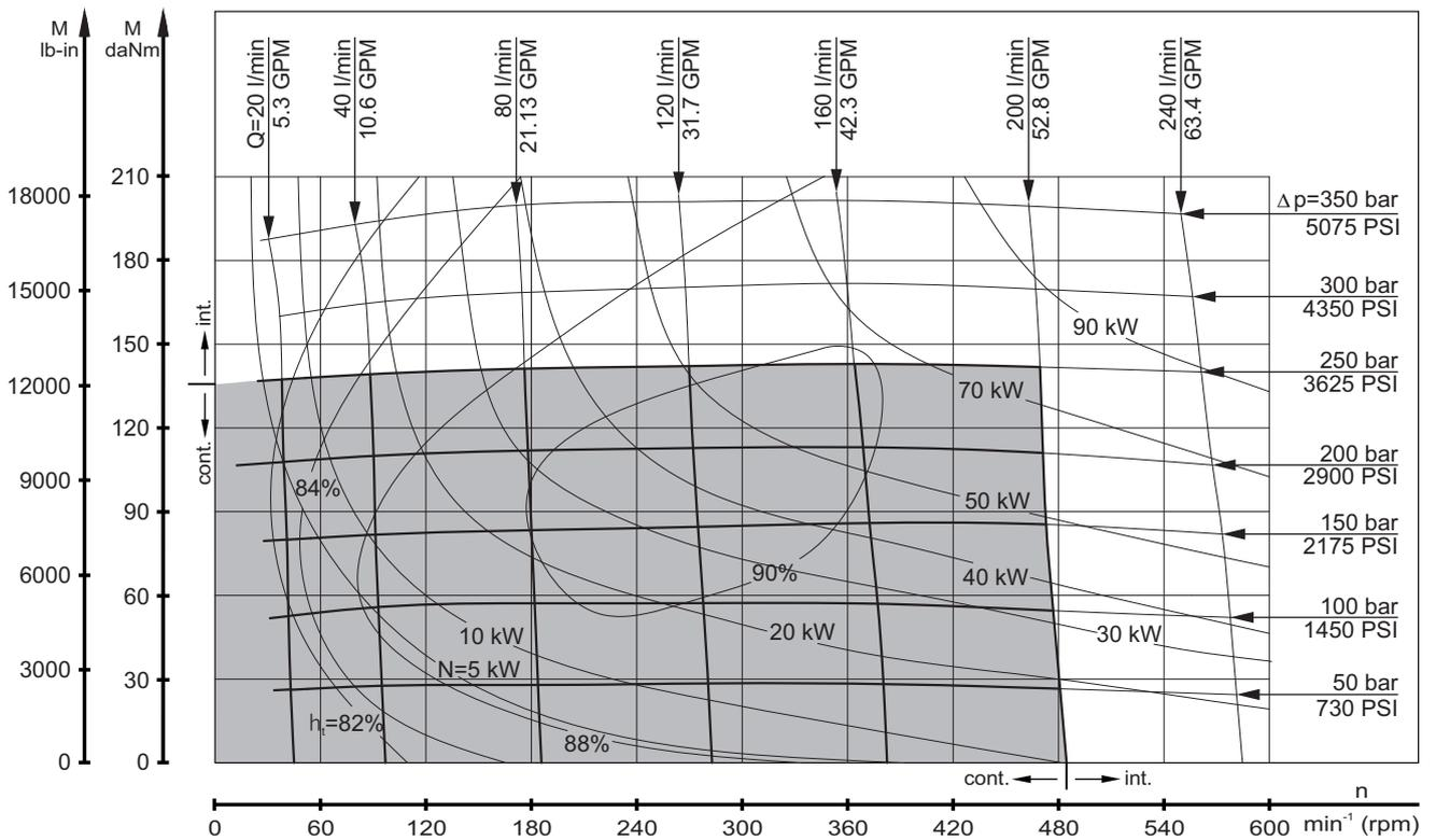
The function diagrams data was collected at back pressure 72.5÷145 PSI [5÷10 bar] and oil with viscosity of 150 SUS [32 mm²/s] at 122°F [50°C].
