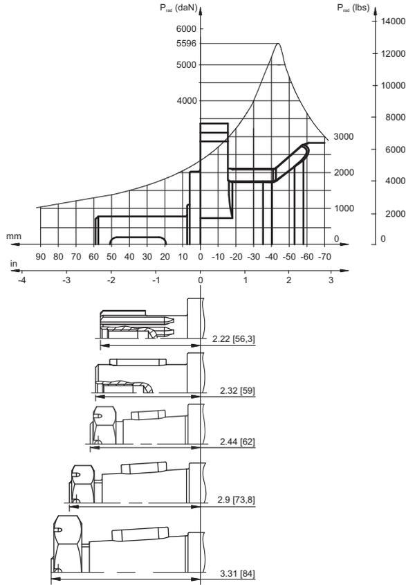
The curves apply to a B10 bearing life (ISO281) of 2000 hours at 100 RPM.
