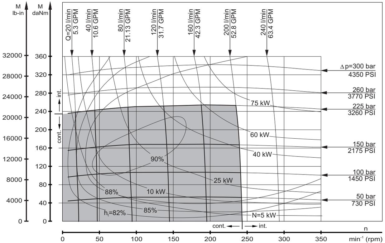
The function diagrams data is for average performance of randomly selected motors at back pressure 72.5÷145 PSI [5÷10 bar] and oil with viscosity of 150 SUS [32 mm<sup>2</sup>/s] at 122°F [50°C].
