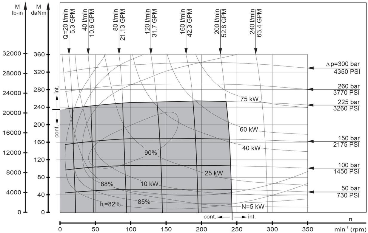
The function diagrams data was collected at back pressure 72.5÷145 PSI [5÷10 bar] and oil with viscosity of 150 SUS [32 mm<sup>2</sup>/s] at 122°F [50°C].
