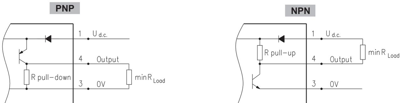
$$R_{Load} [k\Omega] = U_{d.c.} [V] / I_{max} [mA]$$
