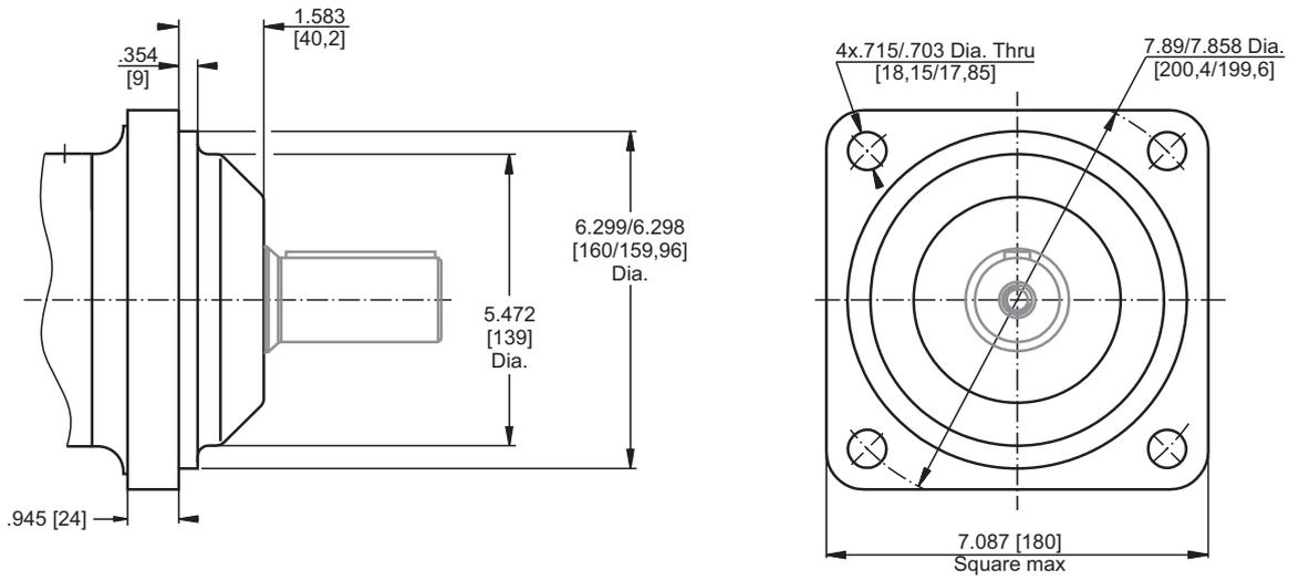
**C** 4-Bolt flange, SAE C mounting flange
