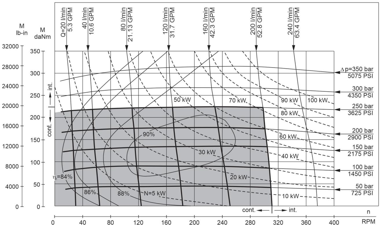
The function diagrams data was collected at back pressure 72.5÷145 PSI [5÷10 bar] and oil with viscosity of 150 SUS [32 mm<sup>2</sup>/s] at 122°F [50°C].
