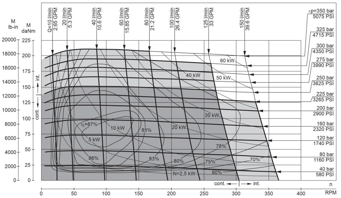
The function diagrams data is for average performance of randomly selected motors at back pressure 72.5÷145 PSI [5÷10 bar] and oil with viscosity of 150 SUS [32 mm<sup>2</sup>/s] at 122°F [50°C].
