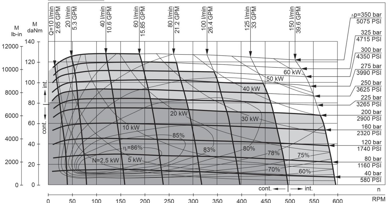
The function diagrams data is for average performance of randomly selected motors at back pressure 72.5÷145 PSI [5÷10 bar] and oil with viscosity of 150 SUS [32 mm<sup>2</sup>/s] at 122°F [50°C].
