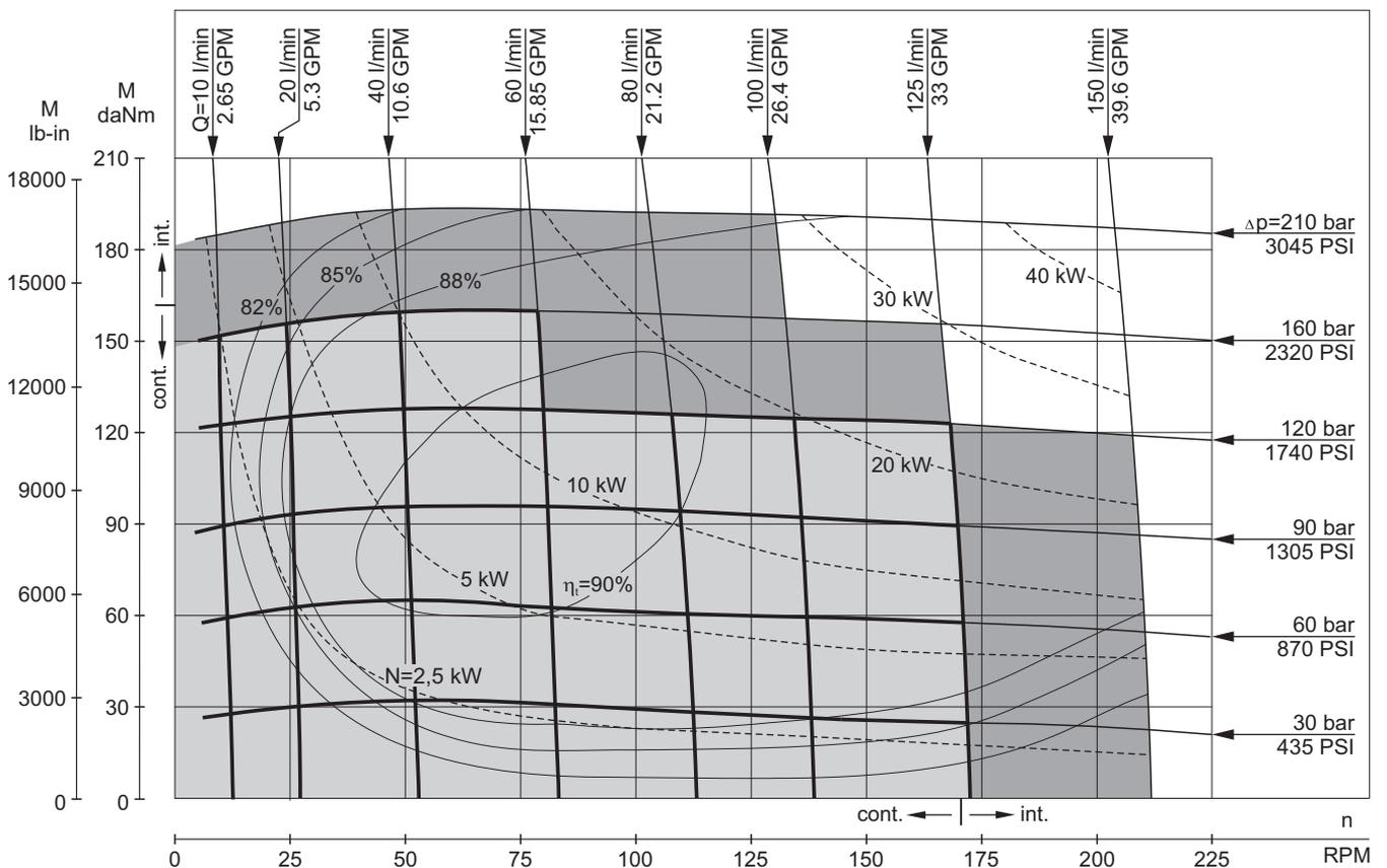
The function diagrams data is for average performance of randomly selected motors at back pressure 72.5 PSI ± 145 PSI [5 ± 10 bar] and oil with viscosity of 150 SUS [32 mm<sup>2</sup>/s] at 122°F [50°C].
